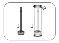
4. Install the set of Filter Sponges. Make sure the sponge is all the way at the bottom of the reactor, flush against the plate - otherwise the media may leak past it when filling.
