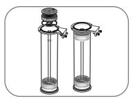
6. Install the other Filter Sponge (not necessary if media diameter is above 2mm) and the upper Media Plate. The plenum may fit snugly, please use caution when sliding it on.
