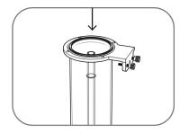
5. Now you can add in your media, taking care not to fill into the central tube. You can temporarily block the top of the central tube to stop media from entering the central tube.
