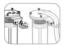
8. Install the hose holder and connect the inlet and outlet hose to the Hose Barbs on the lid.
